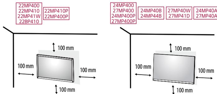
To install the monitor to a wall, attach a wall mounting bracket (optional) to the back of the monitor. Make sure that the wall mounting bracket is securely fixed to the monitor and to the wall.
